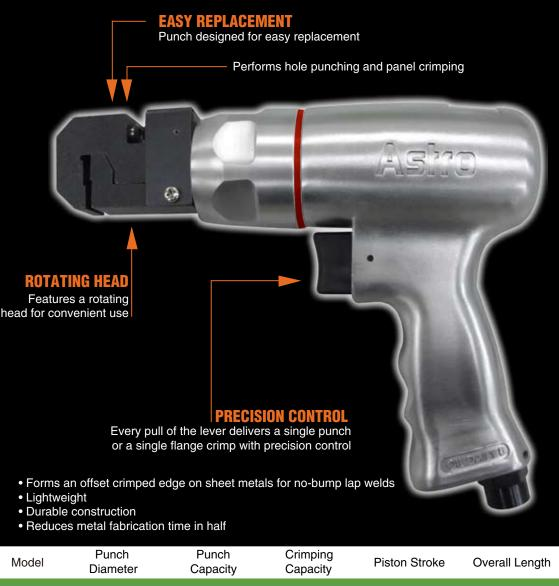
605PT 5.5mm (7/32") 1.6mm (1/16") 5/32" (4mm) 7.87" (200mm) 1.6mm (1/16") Air Inlet Thread Air Hose Avg. Air Net Weight Air Pressure NPT I.D. Size Consumption **SALES AND MARKETING** 90-120psi (6.21-8.28 Bar) 2417 SEAMAN AVENUE 2.47lbs. (1.12kg) 1/4" 3/8" (10mm) 4cfm flat and curved surfaces
